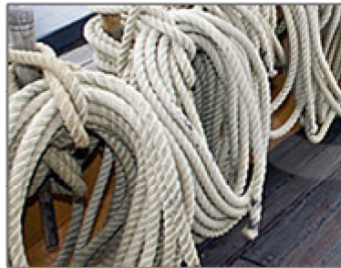
Ropes for making connection with either ship in distress or survival craft (minimum 2)
